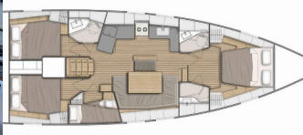
OCEANIS 46.1 - layout 4 CABINS & 2 HEADS
